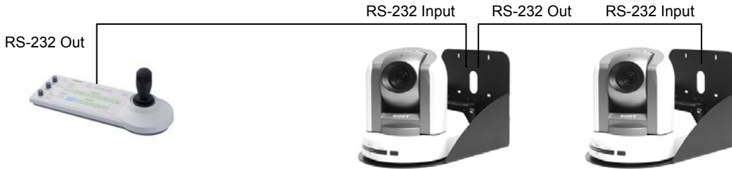
Figure 3: Daisy chain control configuration using two (2) WallVIEW PRO 300 systems and a single RS-232 output control device. See Appendix 1 for wiring and pin-out information.
