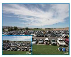
The IP7361 is equipped with a 2-megapixel sensor, making it capable of providing highly detailed images by which users can easily and accurately identify minute objects such as vehicle license plates or facial features.
