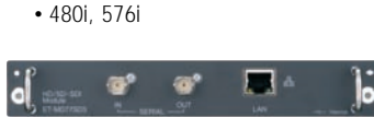
HD/SDI/Network board ET-MD77SD3 • 480i, 576i, 720/60p, 720/50p, 1035/60i, 1080/60i, 1080/50i, 1080/25p, 1080/24p, 1080/24sF, 1080/30p
