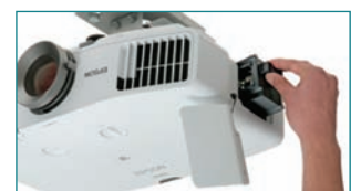
Safe access to lamp
